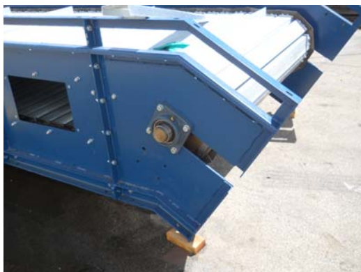
Figure 11 - Bearing support of drive shaft
