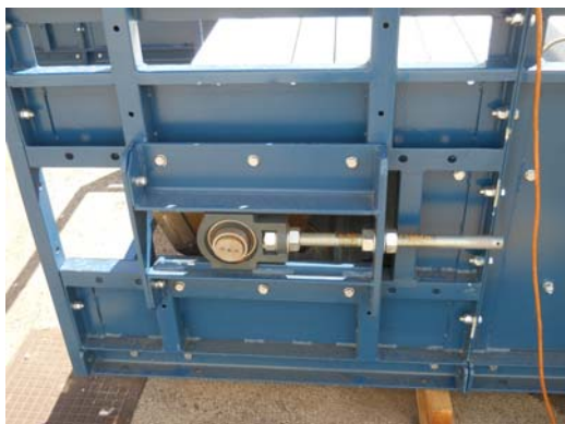
Figure 12 - Bearing support of idle shaft
